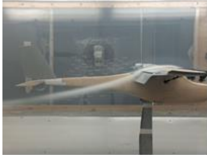
Wake Visualization through smoke generator
