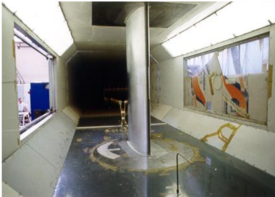
Airfoil 2-D tests
