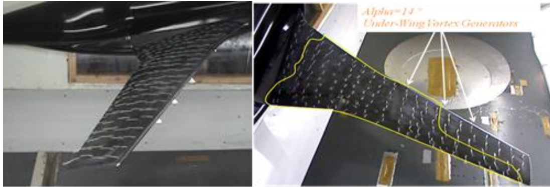
Flow visualization through tufts (stall path detection)
