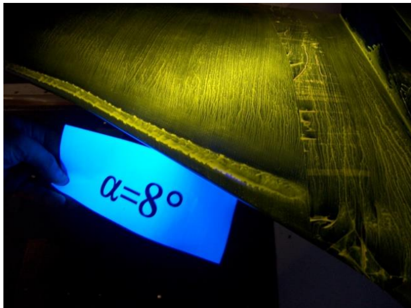
Flow visualization through fluorescent oil Vortex on a 2-D airfoil (left), laminar separation bubble (right)
